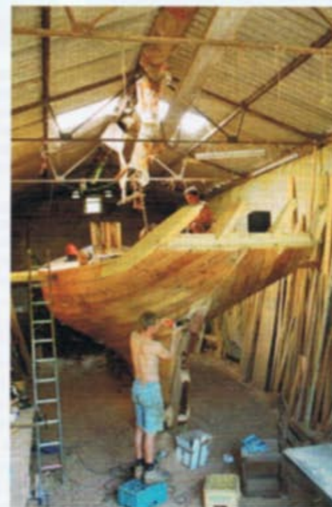
▲ Lucie B 's counter-stern added a considerable amount of time to the build
