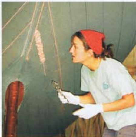
Left: Georgie paying the seams in red-lead putty; Right: Aerial view shows the lovely run of the deck; Below left: Fairing the hull; Below right: Splicing the standing rigging
